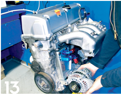
13 Next, install the alternator of your choice, whether it's a B-, D- or K-series unit. The stock lower alternator bolts can also be reused in this kit.
