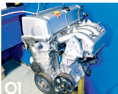
01 The accessory belts are removed from the pulleys, as well as the bolts that secure the water pump to the engine.
