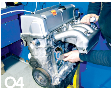
04 The old RTV sealant must be cleaned off the surface of the block. This is a necessary step as any old RTV that's present will cause leaks when the block-off plate is installed.
