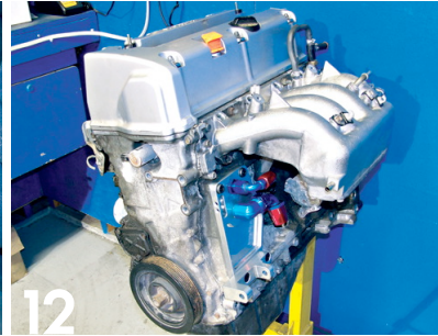
Here is what the block-off plate can look like when quality fittings are used.
