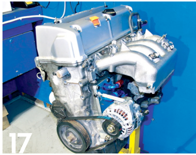
17 The belt that should be used with the kit (which isn't supplied) is a 4PK795, and it can be purchased from any auto parts store.
