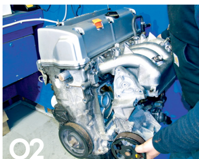
02 Once the bolts in the water pump are removed, the water pump can be removed from the engine. Once the pump assembly is removed, you can see how large this unit is.
