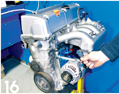
16 Adjust the radius arm so that the alternator moves toward the engine to allow the belt to be installed more easily.
