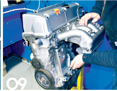
Now, the alternator bracket that is supplied with the kit is installed in the lower bolt location using a pair of M10 40mm bolts.
