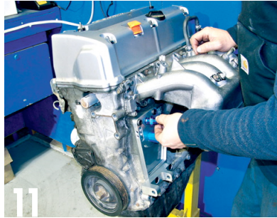
Next, the upper fitting for the vacuum is installed.
