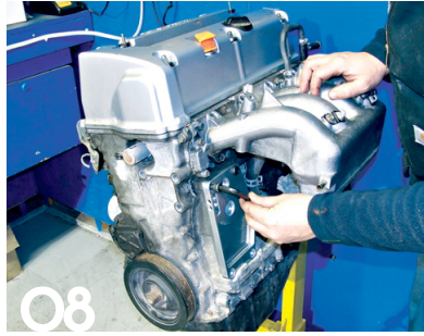
The ETD Racing water pump block-off plate is installed using a pair of M10 30mm bolts in the top holes.
