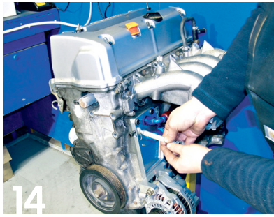
14 At this point, there are two bolts and a spacer left over from the water pump upgrade. The shorter of the two bolts (M8 25mm) is used to secure the radius arm.
