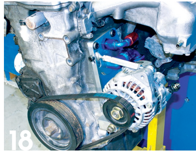
18 The installation is completed, and the engine (???) can be installed into the engine. This upgrade cleans up the engine compartment considerably.
