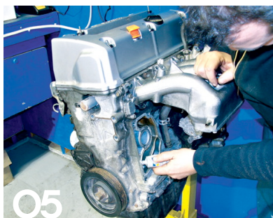
05 Next, the O-ring in the stock water pump assembly is removed as it will be reused as long as it's in good shape.
