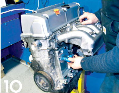
Now, the fittings are to be installed. The first fitting goes into water outlet, and thread sealant is used to prevent leakage.
